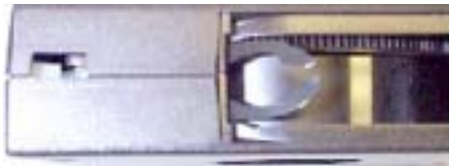
Figure 1-26. Media wrapped too loosely (improper tension)
